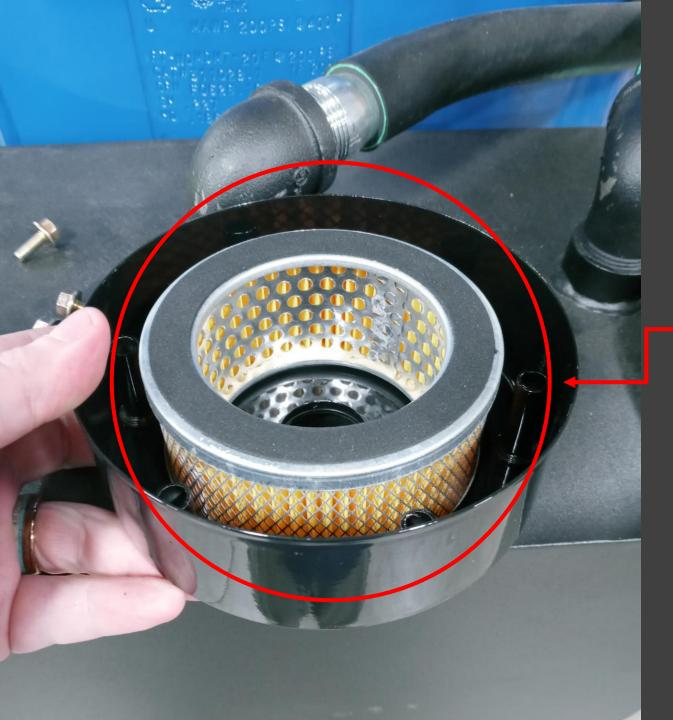
6. Replace filter and reinstall assembly back into Whisper unit ensuring to tighten the wingnut.
